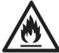
Caution: Risk of fire/ flammable materials
